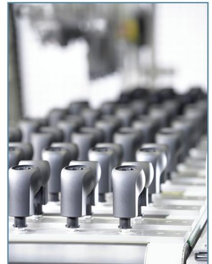
Fig. 1: Gear knobs are produced on ARBURG injection moulding machines (photo: Arburg)
