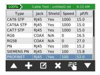
Touch the plus sign ( ) to create a new cable type. Enter the type name and confirm with [Ok]:
