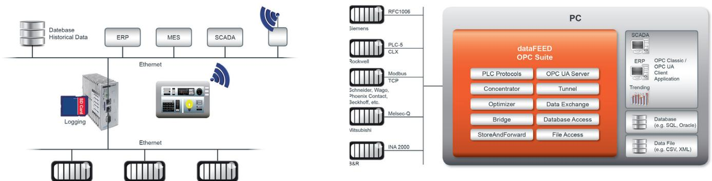
The echocollect e (OPC) product provides an embedded OPC UA Server for easy integration into an overall system (Source: Softing)
