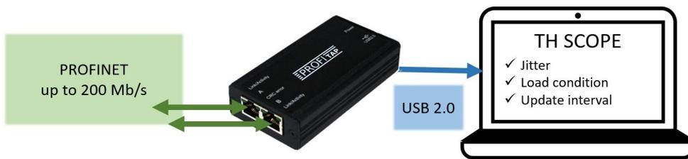
This setup ensures that the frame traffic of each PROFINET device in the network is recorded. What follows is an analysis of the traffic time of the data frames. The measured jitter, load ratio and update intervals are recorded in the acceptance reports.
